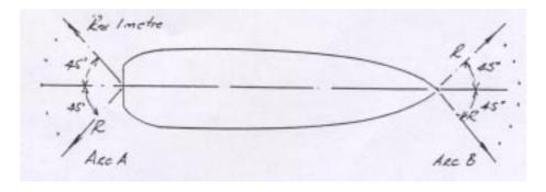
The "near the model" wave measuring probe to be positioned either on arc A or arc B (**Figure a**).
