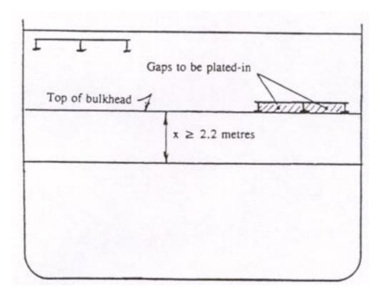
Ship with hanging deck (in way of the barrier)
